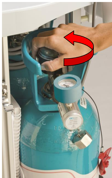
Figure 1 Rotating cylinder handle counter-clockwise
